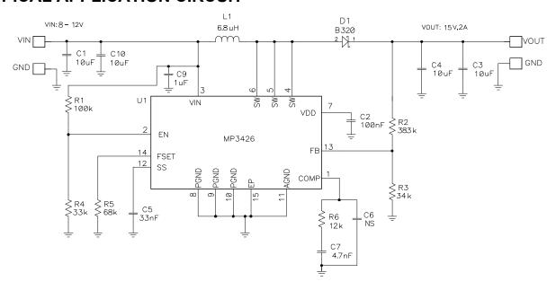
Figure 4: Typical Application Schematic—15V Output
