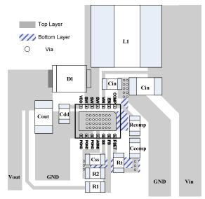
Figure 3: Recommended PCB Layout
