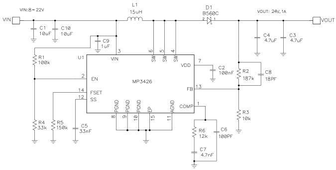
Figure 5: Typical Application Schematic—24V Output
