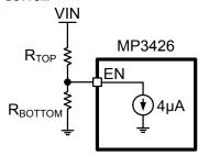
Figure 2: EN Resistor Divider
