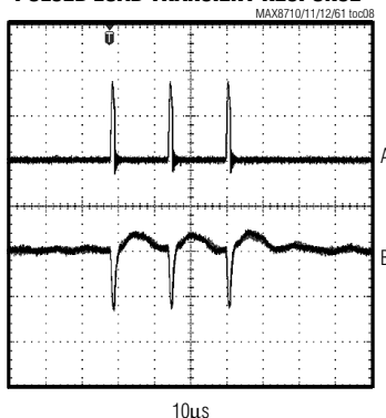
MAX8761 LINEAR-REGULATOR PULSED LOAD TRANSIENT RESPONSE
