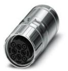
Cable connector, straight long, Screw locking, M40, Number of positions: 2+3+PE, Type of contact: Socket, Crimp connection, Shielded: Yes, Cable cross section: 9 mm...14 mm
