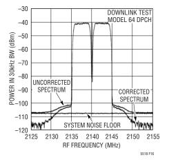
Figure 16. 2-Channel W-CDMA Spectrum
