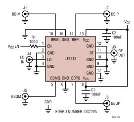
Figure 8. Evaluation Board Circuit Schematic
