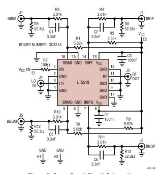
Figure 9. Demo Board Circuit Schematic
