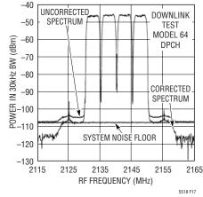
Figure 17. 4-Channel W-CDMA Spectrum
