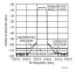
Figure 15. 1-Channel W-CDMA Spectrum
