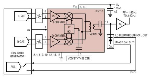
Figure 13. 1.5GHz to 2.4GHz Direct Conversion Transmitter Application with LO Feedthrough and Image Calibration Loop
