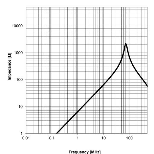
GENERAL TOLERANCE CREATED CHECKED Würth Elektronik eiSos GmbH & Co. KG EMC & Inductive Solutions SSt SSt DIN ISO 2768-1m Max-Eyth-Str. 1 74638 Waldenburg **WE-MAPI SMD Shielded Power** Tel. +49 (0) 79 42 945 - 0 Inductor ORDER CODE www.we-online.com 74438335010 eiSos@we-online.com REVISION STATUS BUSINESS UNIT
