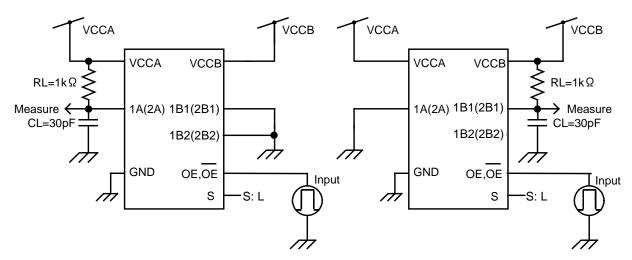
Figure 4 tpLz, tpzL Test Circuits
