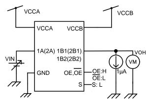
Figure 9 Test Circuit
