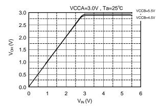
Figure 10 Input/Output Characteristics (Typ.)
