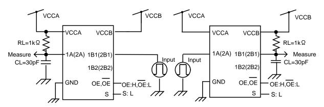
Figure 3 tpLH, tpHL Test Circuits
