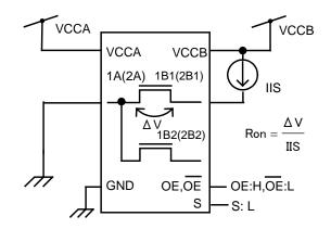
Figure 2 ON-resistance Test Circuits
