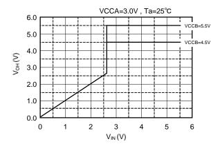
Figure 8 Input/Output Characteristics (Typ.)
