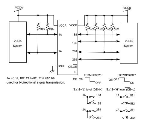
Figure 1 Application Circuit Diagram
