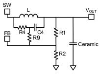
Figure11—Simplified Ceramic Capacitor Circuit
