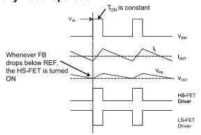
Figure 2—Heavy Load Operation
