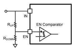
Figure 9—Adjustable UVLO Threshold
