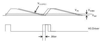
Figure 5—Jitter in Skip Mode
