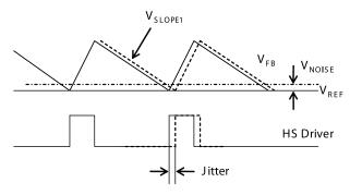
Figure 4—Jitter in PWM Mode
