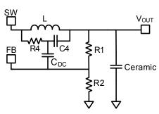
Figure 12—Simplified Ceramic Capacitor Circuit with DC Blocking Capacitor
