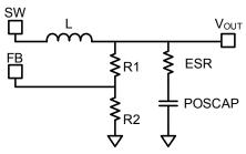
Figure 10—Simplified POSCAP Circuit
