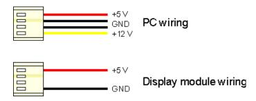
Figure 4: Wiring for 5V Modules
