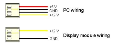
Figure 6: Wiring for 12 Volt Modules
