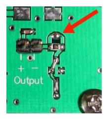
Figure 17: Bypassing 240 ohm Resistor
