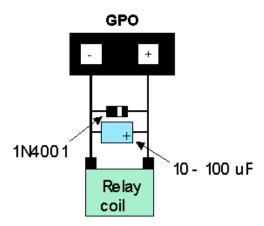
Figure 18: Clamping a Relay
