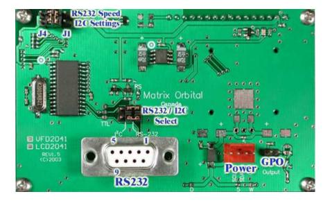
Figure 2: Electrical Connections
