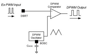
Figure 2—PWM Dimming Method
