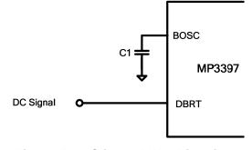
Figure 5—DC input PWM Dimming
