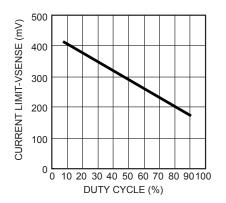
Figure 3—V<sub>SENSE</sub> vs Duty Cycle
