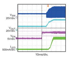
DC Burst Dimming V<sub>PWM</sub> = 0.9V, C<sub>BOSC</sub> = 2.2nF
