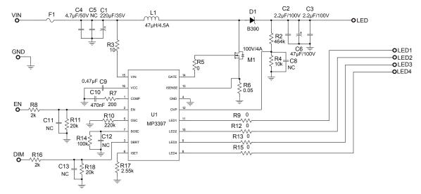
Figure 7—Drive 14 LEDs in Series, 4 Strings 330mA/string,10% D<sub>PWM</sub>
