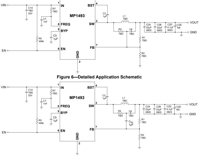
Figure 7—Detailed Application Schematic with Low ESR Ceramic Capacitor and DC Blocking Capacitor.
