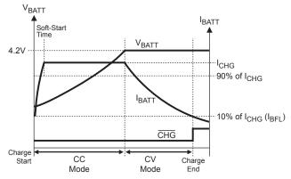
Figure 3—MP2606 Typical Charging Procedure
