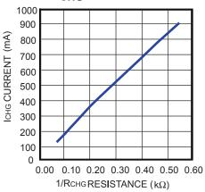
Figure 4—Charge Current vs 1/R<sub>CHG</sub>
