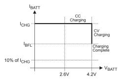
Figure 2—MP2606 Typical Charging Profile
