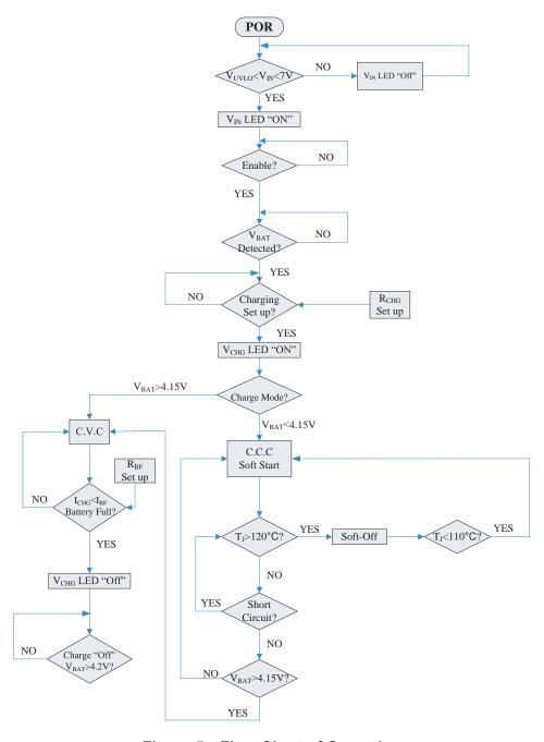
Figure 5—Flow Chart of Operation
