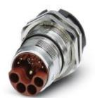
Device connector for rear wall, straight, shielded: yes, Screw locking, M23, No. of pos.: 4+4+4+PE / 3+N+PE, type of contact: Pin, Crimp connection, Flat gasket, Central fastening M26 x 1, Panel thickness min.: 1.5 mm, Panel thickness max.: 5 mm
