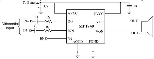
Figure 3—MP1740 Application Schematic with Differential Input
