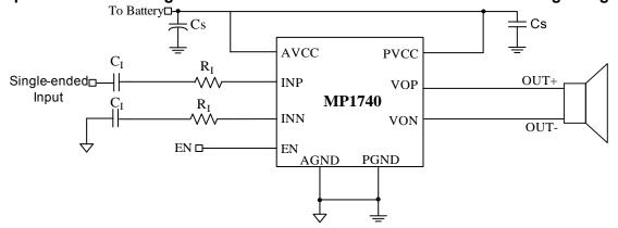
Figure 4—MP1740 Application Schematic with Single-Ended Input
