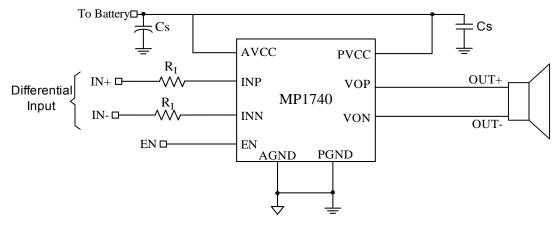
Figure 2—MP1740 Application Schematic with Differential Input
