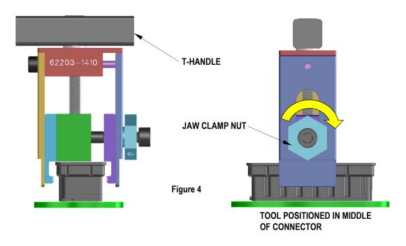
5. To firmly grip the connector, be sure to use the provided wrench to securely tighten the Jaw Clamp Nut. See Figure 5.
