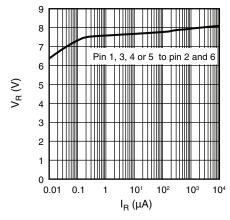
Fig. 5 - Typical Reverse Voltage  $V_{\text{R}}$  vs. Reverse Current  $I_{\text{R}}$
