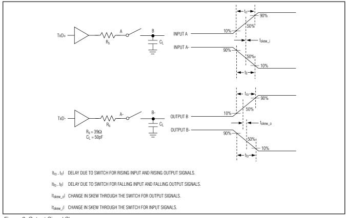
Figure 2. Output Signal Skew
