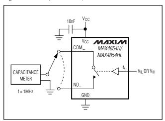
Figure 5. Channel Off-/On-Capacitance
