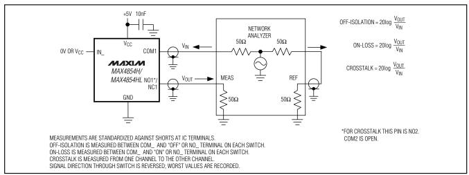
Figure 4. On-Loss, Off-Isolation, and Crosstalk
