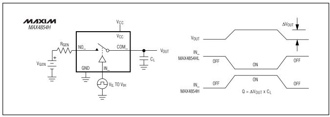
Figure 3. Charge Injection
