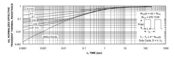
Figure 11. Transient Thermal Response Curve.
