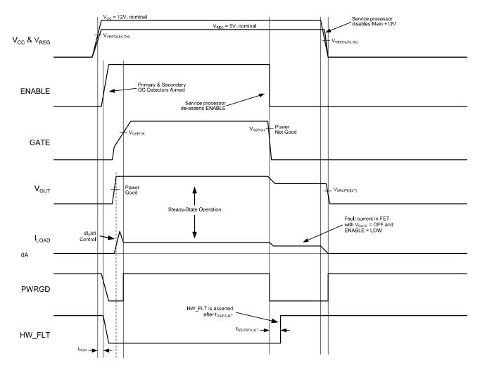
Figure 9. Hardware Fault by a MOSFET DS Short after Steady-State Operation (ENABLE = HIGH-to-LOW)
