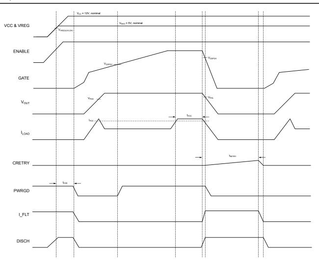
Figure 6. Primary Overcurrent Fault with Auto-Retry to Reset the Circuit Breaker
