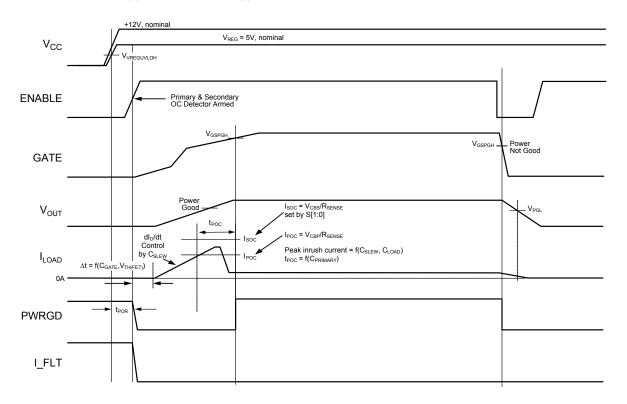
Figure 2. Basic Startup Cycle
