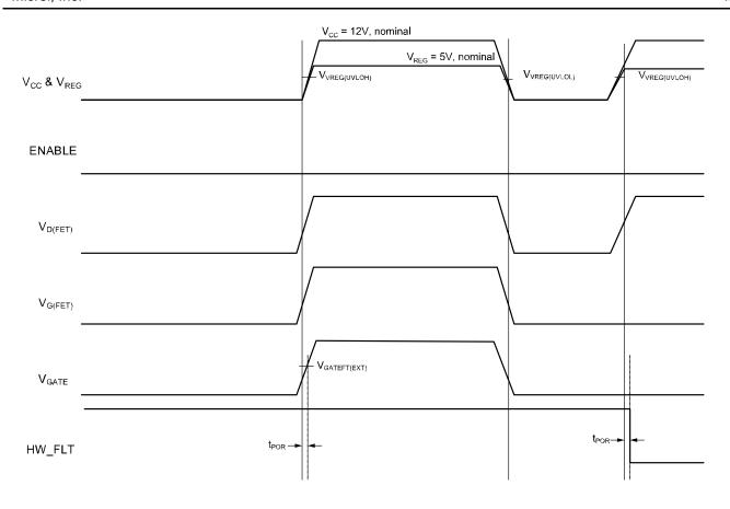
Figure 7. Hardware Fault Detection of a MOSFET DG Short with ENABLE = LOW
