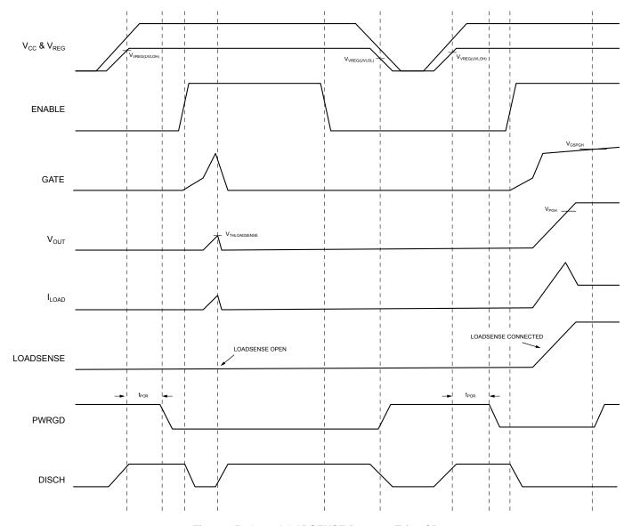
Figure 15. Open LOADSENSE Detector Trips CB
