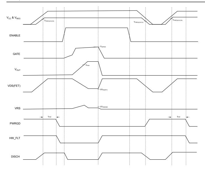
Figure 11. Shorted  $R_{\text{SENSE}}$  Trips Circuit Breaker and Asserts HW\_FLT
