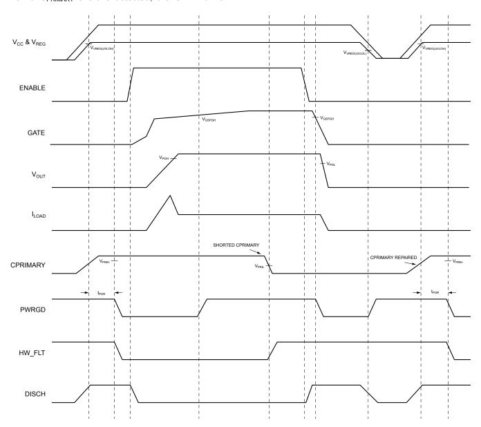
Figure 13. Shorted CPRIMARY Detector Asserts HW\_FLT During Steady-State
