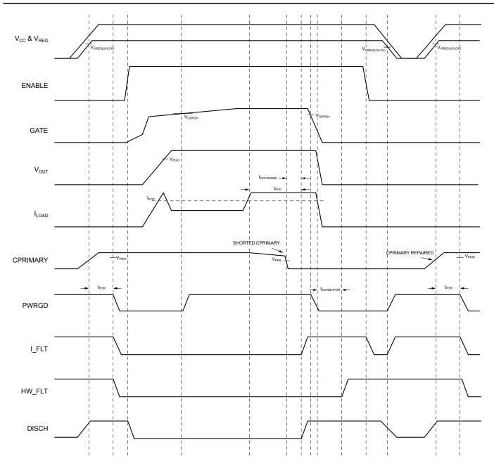
Figure 14. Shorted  $C_{\text{PRIMARY}}$  Detector Asserts HW\_FLT after Primary OC Event
