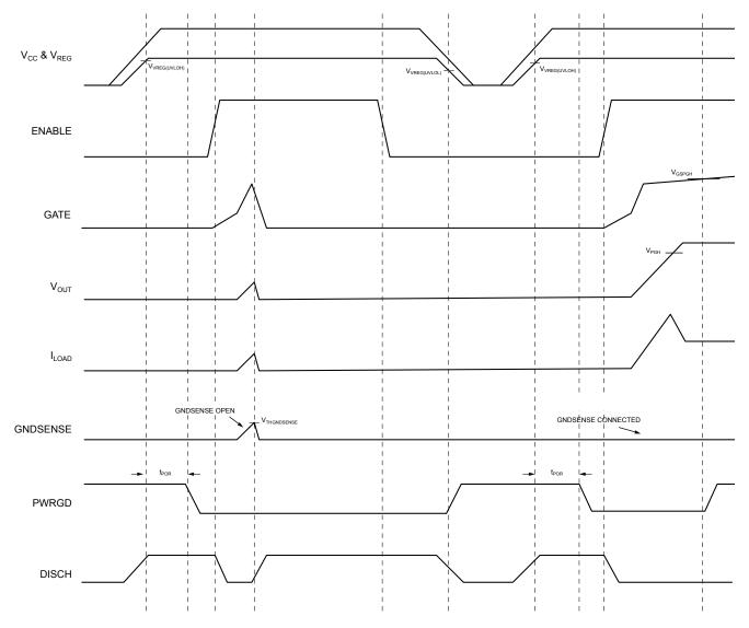
Figure 16. Open GNDSENSE Detector Trips CB
