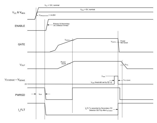
Figure 4. Secondary OC Detector Trips Circuit Breaker
