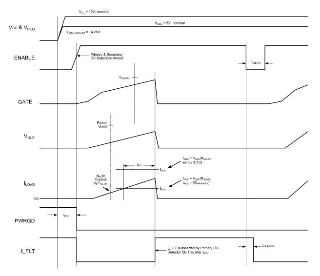
Figure 5. dlp/dt Load Charge Profile w/ Primary OC Circuit Breaker (CB) Trip w/ CB Reset
