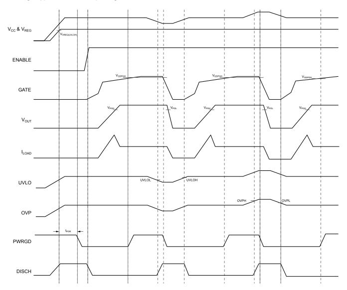
Figure 17. UVLO and OVP Operation
