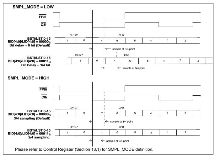
Figure 9 - Backplane and Local Input Bit Delay or Sampling Point Selection Timing Diagram for Data Rate of 32Mbps
