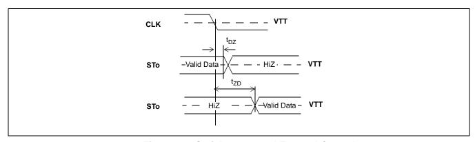
Figure 21 - Serial Output and External Control
