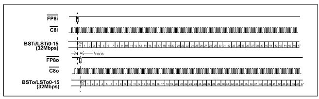
Figure 7 - Input and Output (Generated) Frame Pulse Alignment for Different Data Rates
