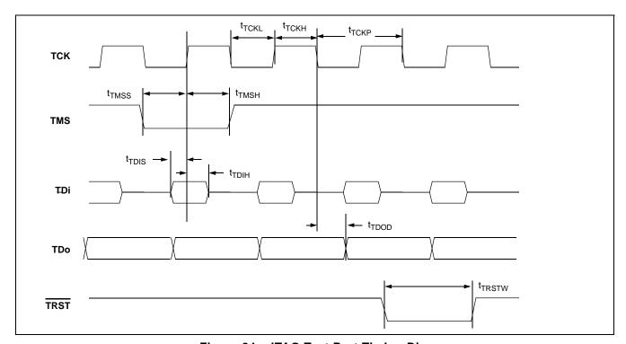
Figure 24 - JTAG Test Port Timing Diagram
