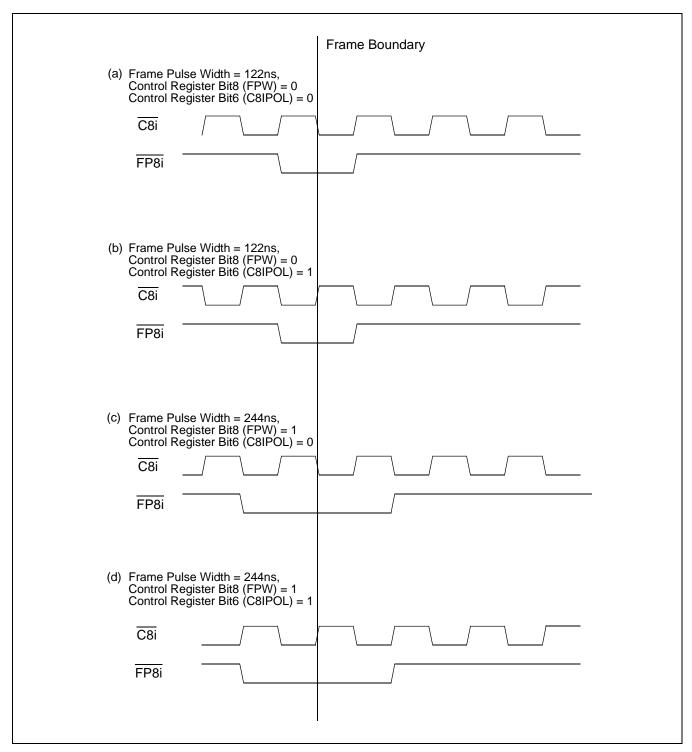
Figure 15 - Frame Boundary Conditions, ST-BUS Operation
