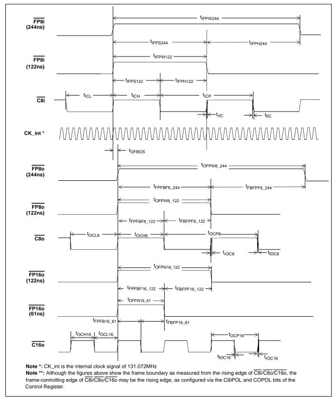
Figure 18 - Input and Output Clock Timing Diagram for GCI-Bus
