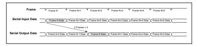
Figure 11 - Data Throughput Delay with Input Ch0 Switched to Output Ch0
