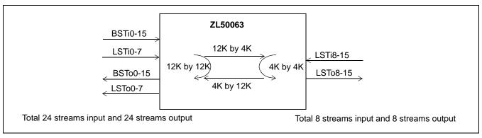
Figure 5 - 12,288 by 4,096 Channels Blocking Bi-directional Configuration
