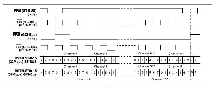
Figure 6 - ST-BUS and GCI-Bus Input Timing Diagram
