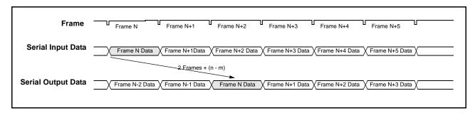
Figure 12 - Data Throughput Delay with Input Ch0 Switched to Output Ch13
