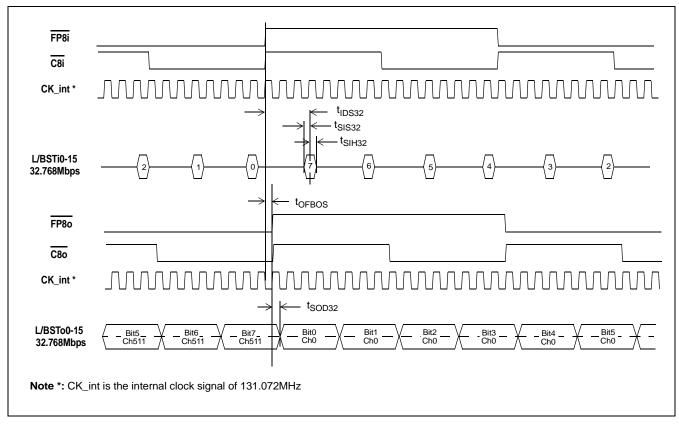
Figure 20 - GCI-Bus Local/Backplane Data Timing Diagram (32Mbps)
