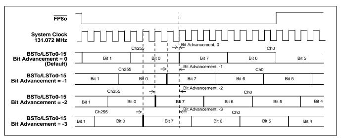
Figure 10 - Local and Backplane Output Advancement Timing Diagram for Data Rate of 32Mbps
