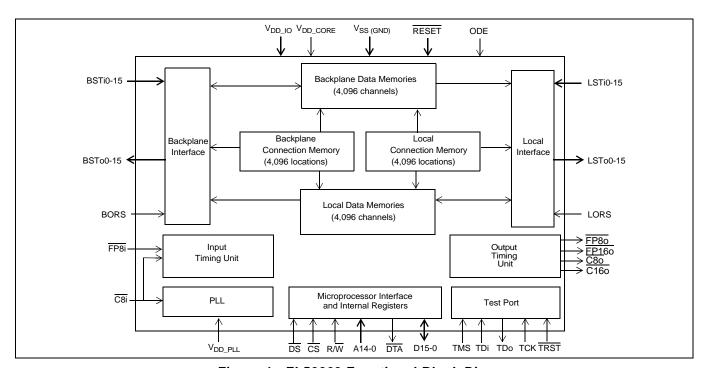
Figure 1 - ZL50063 Functional Block Diagram
