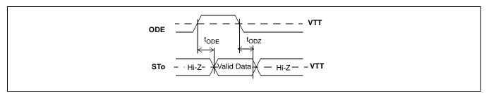
Figure 22 - Output Driver Enable (ODE)
