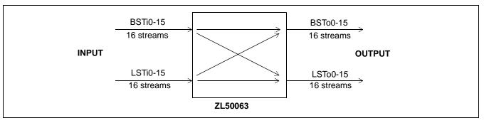
Figure 3 - 16,384 x 16,384 Channels (32Mbps), Unidirectional Switching
