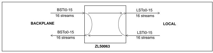
Figure 4 - 8,192 x 8,192 Channels (32Mbps), Bi-directional Switching
