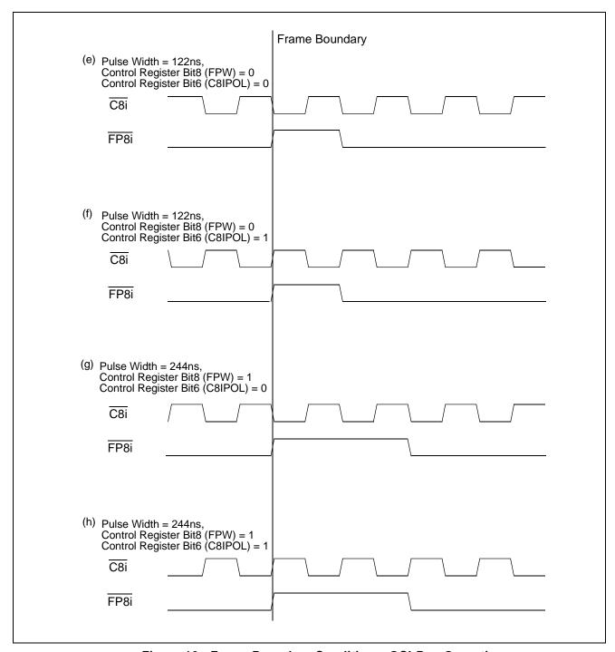
Figure 16 - Frame Boundary Conditions, GCI-Bus Operation
