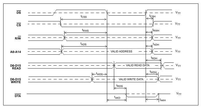
Figure 23 - Motorola Non-Multiplexed Bus Timing
