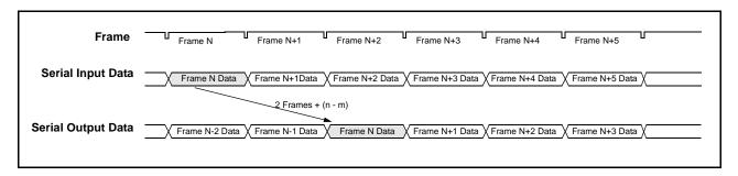
Figure 13 - Data Throughput Delay with Input Ch13 Switched to Output Ch0
