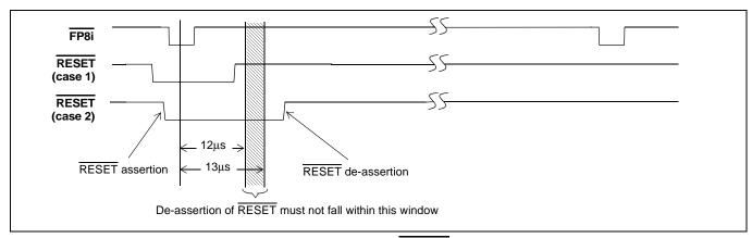
Figure 14 - Hardware RESET De-assertion
