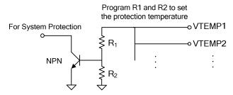
Figure 4: System Thermal Protection PCB Layout Guide Line
