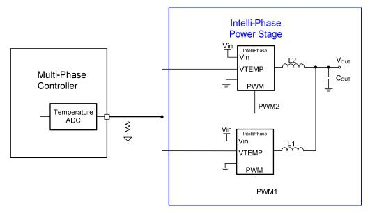
Figure 3: Multi-Phase Temperature Sense Utilization
