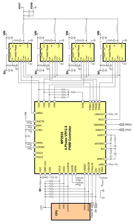
Figure 5: 4-Phase Intelli-Phase with MP2935 VR12.5 Controller
