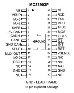
Note: MC33903D, MC33903S, and MC33903P are footprint compatible.
