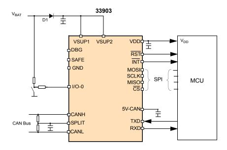
Figure 4. 33903 simplified application diagram
