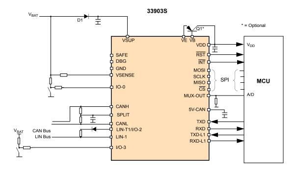
Figure 6. 33903S simplified application diagram
