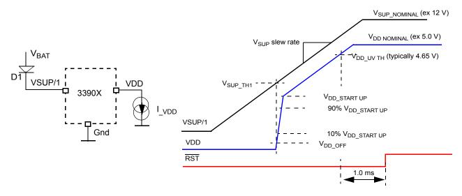
Figure 28. V<sub>DD</sub> start-up versus V<sub>SUP/1</sub> tramp
