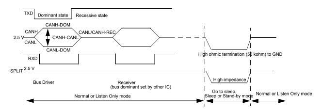
Figure 34. Bus signal in TXD/RXD and LP mode
