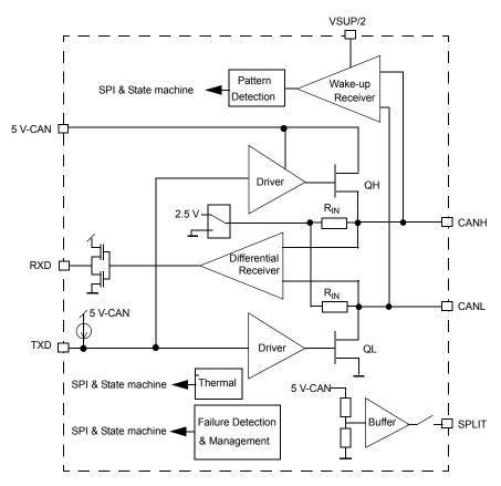
Figure 33. CAN interface block diagram
