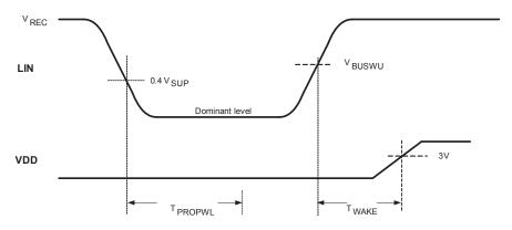
Figure 20. LIN wake-up LP  $V_{\text{DD}}$  off mode timing
