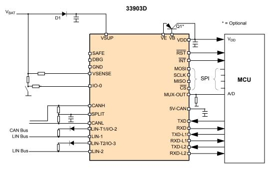
Figure 5. 33903D simplified application diagram
