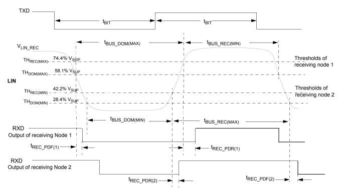
Figure 18. LIN timing measurements for normal slew rate
