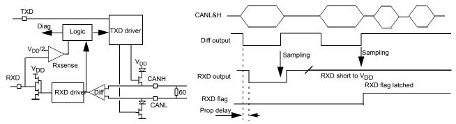
The RXD flag is not the RXPR bit in the LPC register, and neither is the CANF in the INTR register.
