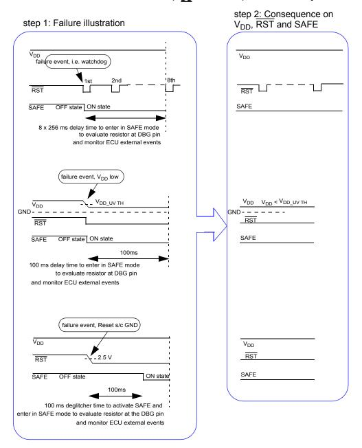
Figure 31. SAFE mode A behavior illustration
