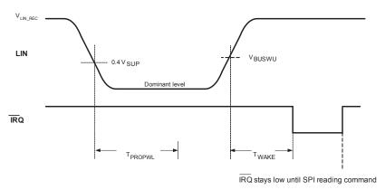
Figure 21. LIN Wake-up LP  $\mathbf{V}_{\mathrm{DD}}$  ON Mode Timing
