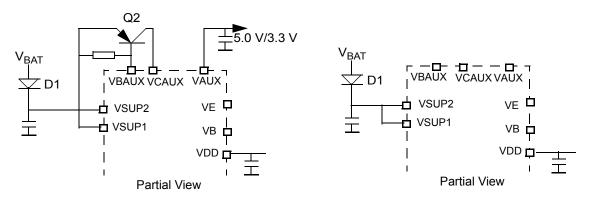
ex 3: No External Transistor,  $V_{DD}$  ~100 mA Capability delivered by internal path transistor.
