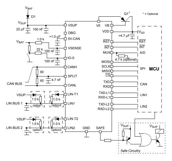
58. Tested per specific OEM EMC requirements for CAN and LIN with additional capacitor > 10  $\mu$ F on VSUP pin
