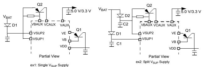
Optimized solution for cranking pulses. C1 is sized for MCU power supply buffer only.
