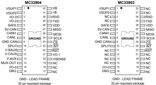
Note: MC33905D, MC33905S, MC33904 and MC33903 are footprint compatible,
