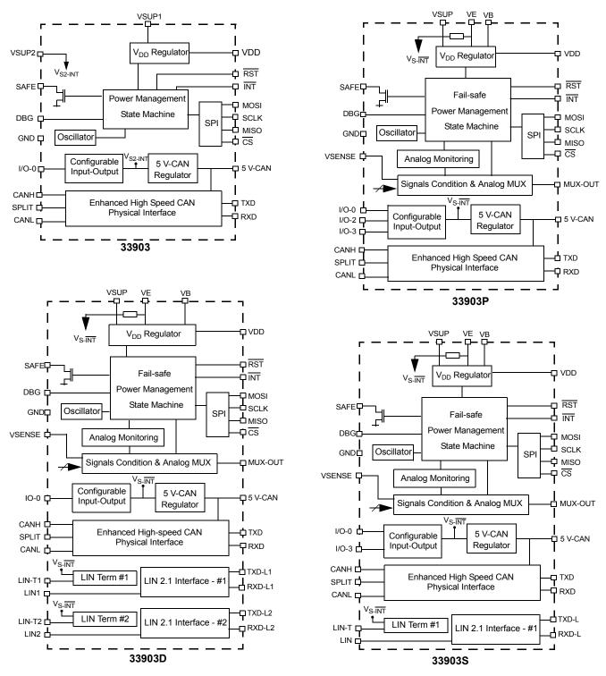
Figure 10. 33903 internal block diagram
