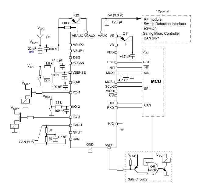
56. Tested per specific OEM EMC requirements for CAN and LIN with additional capacitor > 10  $\mu\text{F}$  on VSUP1/VSUP2 pins
