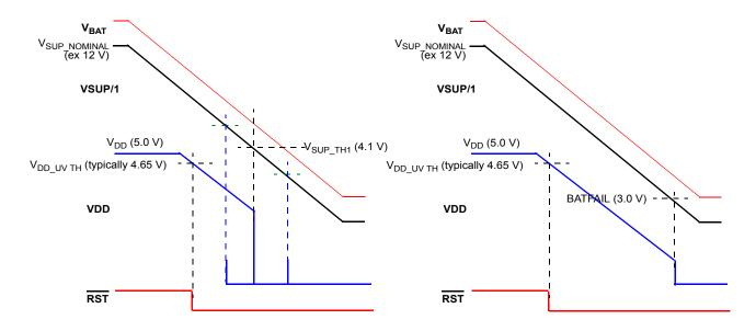
Case 3: "V<sub>DD UV TH</sub> 4.6V", with bit Crank = 0 (default value)
