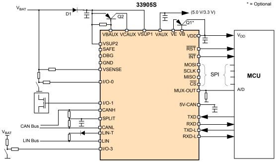
Figure 2. 33905S simplified application diagram
