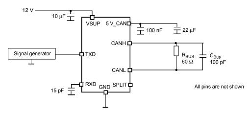
Figure 17. Test circuit for CAN timing characteristics
