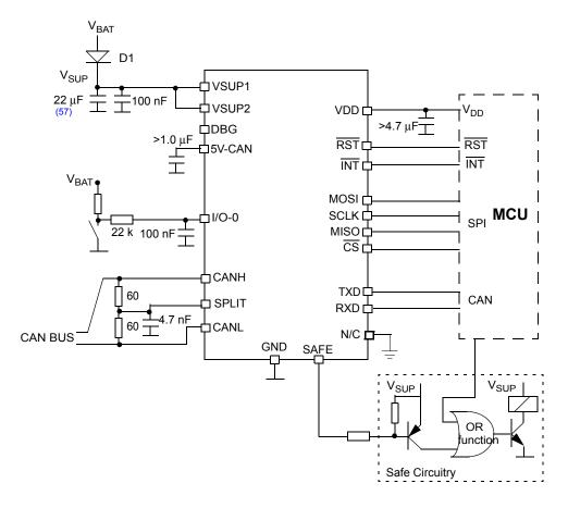
57. Tested per specific OEM EMC requirements for CAN and LIN with additional capacitor > 10  $\mu$ F on VSUP1/VSUP2 pins
