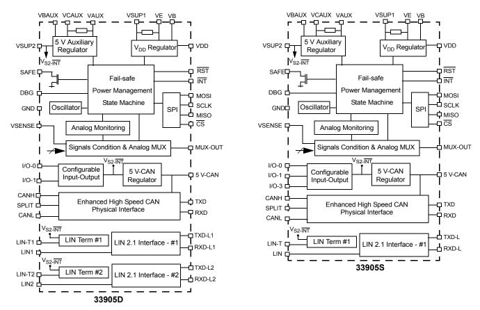
Figure 8. 33905 internal block diagram
