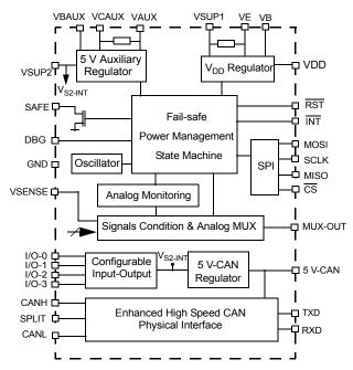
Figure 9. 33904 internal block diagram
