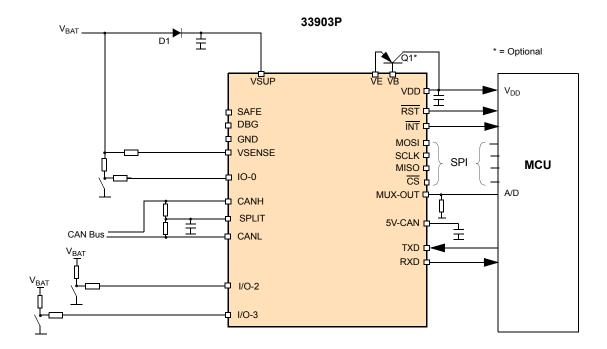
Figure 7. 33903P simplified application diagram
