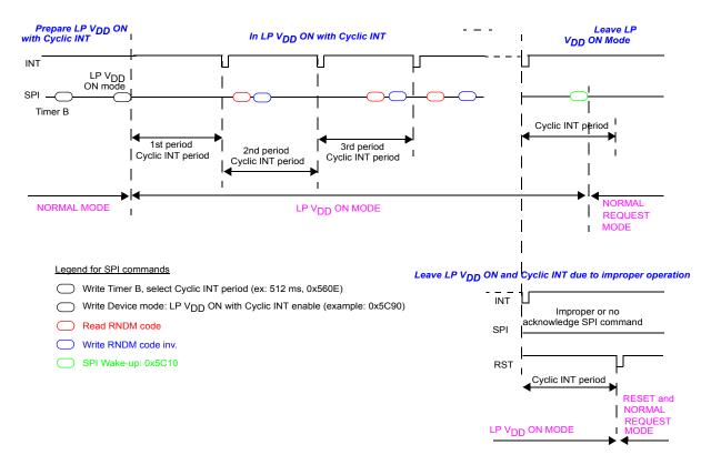
Figure 27. Cyclic interrupt operation
