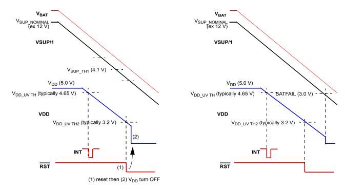
Case 5: "V<sub>DD UV TH</sub> 3.2V", with bit Crank = 0 (default value)
