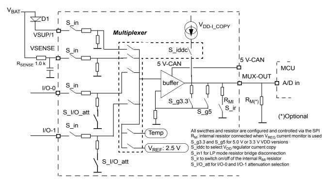
Figure 22. Analog multiplexer block diagram
