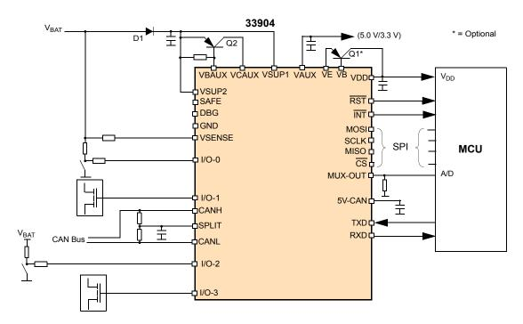
Figure 3. 33904 simplified application diagram
