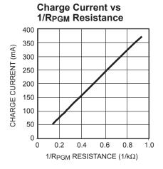
Figure 3—Charge Current vs. 1/R<sub>PGM</sub> Resistance
