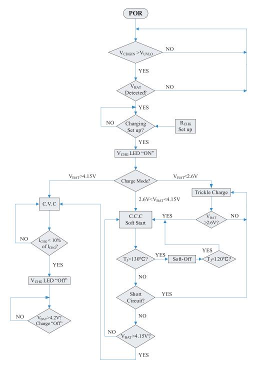
Figure 5—Flow Chart of Charger Operation
