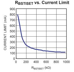
Figure 4—BSTISET Resistance vs. BSTSW Current Limit
