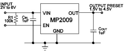
Figure 2 —MP2009 Typical Application Circuit
