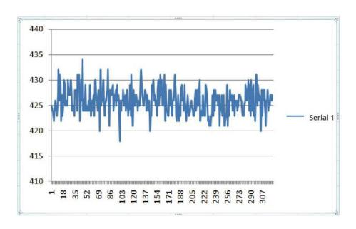
Figure 14 Measuring volatility when true value is 423cm
