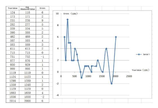
Figure 12 Error performance of outdoor measurement
