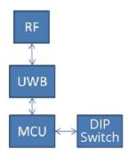
Figure 4 Hardware system of PK-1000 anchor
