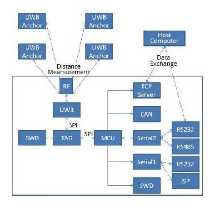
Figure 3 Hardware system of PK-1000 tag
