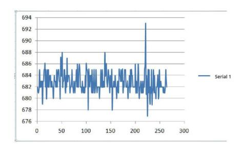
Figure 13 Measuring volatility when true value is 679cm
