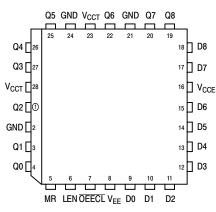
Figure 1. PLCC-28 Pinout (Top View)
