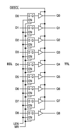
Figure 2. Logic Diagram
