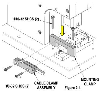
11. Install the cable mounting clamp bracket by positioning the bracket over the two mounting holes. See Figure 2-4. Then
