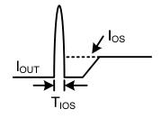
Figure 2—Short Circuit Response Time
