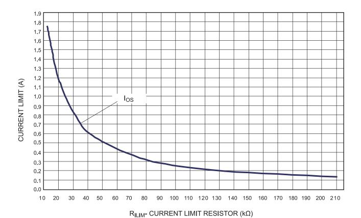
Figure 5—Current-Limit vs RILIM
