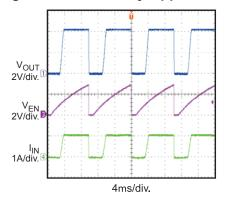
Figure 7—Auto-Retry Waveform
