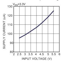
**Supply Current, Output Disabled vs. Input Voltage**
