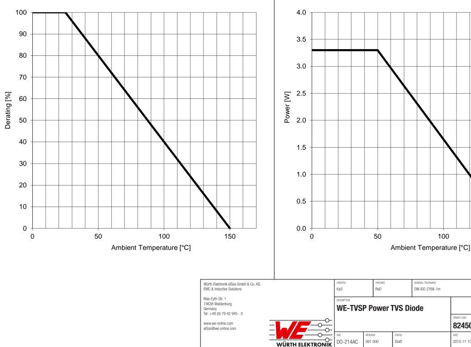
**Steady State Power Dissipation Derating**
