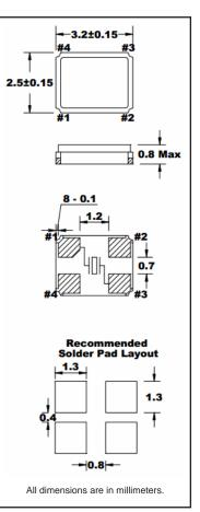
Note: Dimensional drawing is for reference to critical specifications defined by size measurements. Certain non-critical visual attributes, such as side castellations, etc. may vary. The above specifications, having been carefully prepared and checked, is believed to be accurate at
