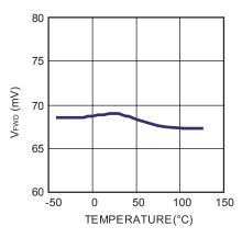
Turn off threshold vs. Temperature
