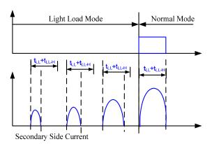
Figure 6: MP6903 Exits Light Load Mode
