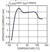
Light Load Mode Current vs. Temperature
