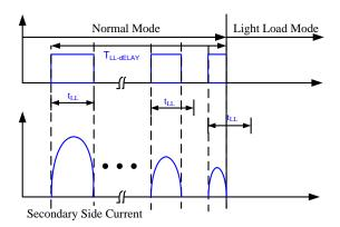
Figure 5: MP6903 Enters Light Load Mode
