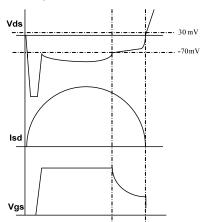
Figure 3: Synchronous Rectification
